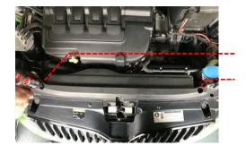
6 Remove the 8 x T25 bolts from the airbox lid and remove the OE air filter.
