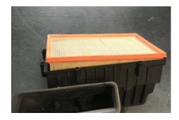
7 Remove the snow/mud filter from the bottom of the airbox by using a flat headed screwdriver to release the tabs around the outside.
