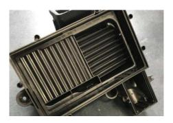
8 Fit the Revo air filter (supplied) into the airbox, refit the 8 x T25 bolts and tighten to the factory torque specification.
