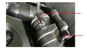
2 Remove the hose clamp from the intake hose and then pull the vacuum hose free from its clip and move out of the workspace.
