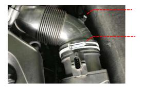
3 Using a 7mm socket, loosen the hose clamp that secures the intake hose onto the turbo inlet and remove the intake hose from the vehicle. Next, unclip the 2 x wiring looms that are attached to the hose and position out of the workspace.
