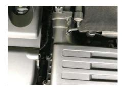
11 Fit the Revo intake hose, make sure the 2 x hose clamps are in a good location for access and then tighten to 5Nm.
