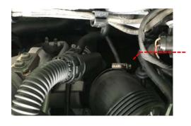
4 Remove the airbox assembly by pulling firmly upwards to free from the 3 x rubber grommets.
