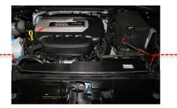
8 Reinstall the airbox, as removed, pushing onto the rubber mounting grommets.
