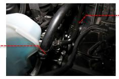
7 Install the new Revo carbon front section as shown and secure using the 2 x M5x15 bolts (supplied) into the existing holes where the OE screws were.
