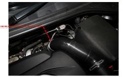
Pull off the vacuum pipe form the airbox, then pull up on the airbox to remove from the rubber mounts.
