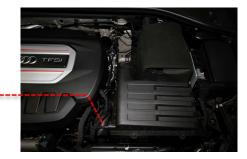
Remove the 2 x screws holding the front section in place then unclip from the tabs and remove.
