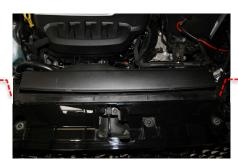
4 Note: if your car is NOT a Golf R or S3 then move to step 7. Remove 2 x two self-tapping screws holding the coolant pipe on the back of the radiator.
