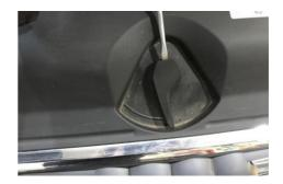
2 Remove the slam panel by unclipping along the front edge and then sliding it out from under the front air scoop.
