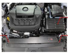
6 Install the machined PCV adapter to the silicone hose using the 25-40mm hose clamp. Next install the Revo machined turbo inlet adapter to the turbo ensuring both o-rings are seated correctly. Once installed you can finally install the new silicone hose using the 70-90 and 60-80 hose clamps to secure. Re-connect the PCV pipe to the take off and the MAF wire to the housing and check everything is tight.
