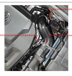
Remove the airbox from the car by first pulling the breather pipe off the lid then pulling airbox up and off the rubber mounts. Next remove the lid loosening the 8 T25 screws. Once removed take the large particle filter out of the bottom of the airbox using a flathead screwdriver. Once you have removed this you can install the new Revo hi-flow panel filter in place and screw the lid back to the base.
