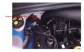
5 Locate the Revo turbo intake hose (larger of the two silicone hoses included in the kit). Double check that the machined breather coupler is installed into the hose and the hose clamp is tight. Loosely install a 60-80 hose clamp onto the smaller end of the Revo turbo intake pipe and install the pipe onto the turbo. Do not tighten the hose clamp at this stage.
