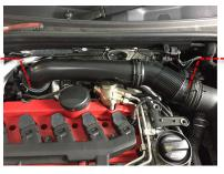
4 Remove the rubber joiner on the turbo held on by another hose clamp. Note: retain this clamp for the install of the Revo intake kit.
