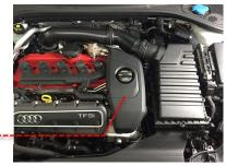
2 Remove the  $2 \times T30$  bolts holding the intake pipe down at the
