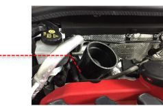
9 Install the new Revo air filter into the airbox.
