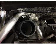
Unclip the vacuum pipe from the airbox and then remove the airbox lid. Once removed take out the OE air filter.
