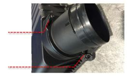
7 Install the new Revo aluminium machined insert onto the airbox lid using the 2 x T25 screws previously removed.
