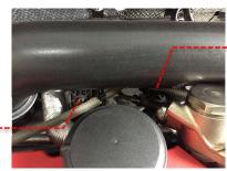
Remove the 2 x hose clamps on the turbo and airbox, then remove the pipe from the car.
