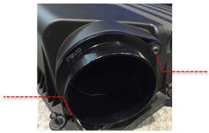
8 Install the Revo turbo intake coupler onto the turbo using the hose clamp you removed earlier.
