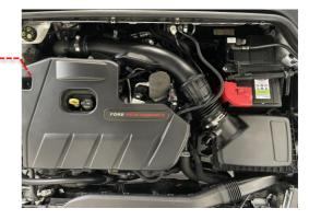
2 Remove the OE intake pipe, loosen the 2 x hose clamps then unclipe the front breather pipe and DV hose to the rear. Finally remove the 2 x 8mm bolts on the bracket and pull away from turbo hose and airbox.
