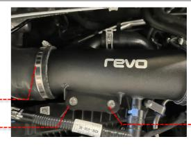
6 Install the new Revo panel filter by unclipping the two clips on top of the airbox, remove the OE paper filter and replace with Revo Hi-Fow version. Re-attach the lid by aligning tabs at side of airbox and then clamping in place with the two clips.
