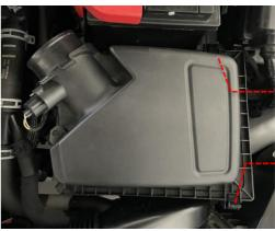
7 Install the new Revo OEM+ intake hose onto the hard pipe and airbox using the supplied 70-90 hose clamps. Check all clamps are tight and OE connections are back in place. Re-install the engine cover reverse of removal.
