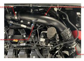
3 Remove the OE turbo inlet pipe by loosening the hose clamp at the turbo end.
