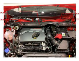
4 Remove the engine cover by pulling up on it and popping it off its locating pins. Then remove the front intake hose by loosening the 2 x hose clamps with a 7mm socket.
