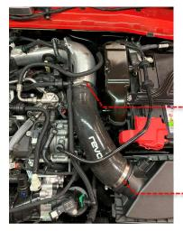
Reattach the two take-offs on the top of the Revo hard pipe and then reconnect the breather pipe to the take-off on the Revo turbo hose at the top of the engine.
