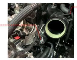
8 Move the coolant reservoir to one side to allow access to the lower intake hose. Do this by removing the tank off the two clips, shown, and place towards the front of the engine.
