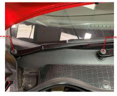
Remove the plenum chamber cover by popping off the 5 x insert clips with a trim tool or flat head screwdriver. Then remove the panel by unclipping from the base of the windscreen.
