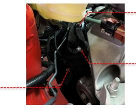
11 Install the breather hose connector into the Revo turbo intake hose, as shown, using the 12-22 hose clamp. Then install onto the turbo inlet pipe using a 60-80 hose clamp. Do not fully tighten yet, to allow for correct alignment first.
