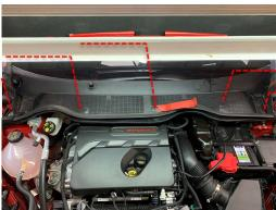
3 Remove the next section by removing the 5 x 10mm bolts, unclip the vacuum line from the underside and then lift the panel from the vehicle.
