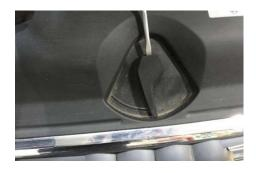
Remove the slam panel by unclipping along the front edge and then sliding it out from under the front air scoop.
