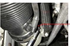
7 Loosen the hose clamp on the turbo intake and pull the hose free.
