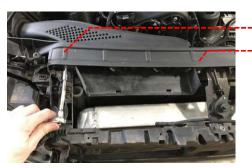
4 Unclip the intake ducting along the front edge and pull free from the airbox.
