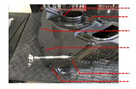
10 Remove the OE air filter by turning anticlockwise.
