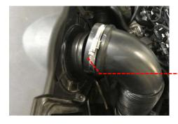
6 Remove the vacuum line attached to the intake hose by pulling gently. Then remove the vacuum line from the engine in the same way and place out of the workspace.
