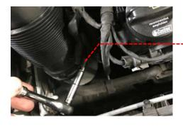
8 With the intake hose removed the OE airbox can be removed by pulling it firmly upwards to release from its 3 x rubber grommets.
