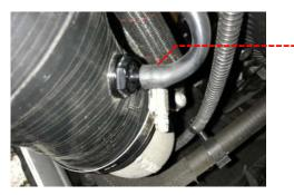
15 Fit the Revo intake hose onto the airbox, making sure it sits correctly. Once this is confirmed tighten both hose clamps and check the fitment.
