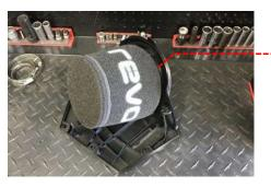
12 Refit the airbox lid and air filter assembly to the bottom of the OE airbox and tighten the 6 x T25 bolts. Visually inspect around the edge of the lid to ensure a good fit and seal.
