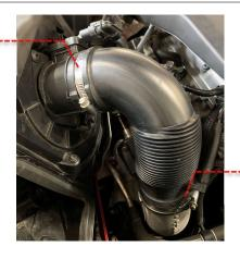
6 Next, disconnect the MAF sensor from the airbox by unclipping the plug from the body and place to the side. Then loosen the 6 x T25 bolts that hold the airbox lid to the base and remove from car.
