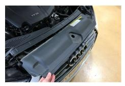
Remove the 2 x T25 bolts from the intake ducting.
