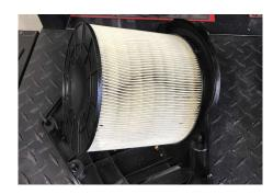
8 Install the new Revo air filter to the airbox lid in the same method as removal.
