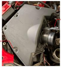
$7\,$   $\,$  Remove the OE air filter by turning anticlockwise.
