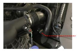
3 Using a 7mm socket, loosen the hose clamp that secures the intake pipe to the airbox.
