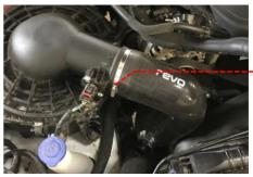
11 Refit the breather hose onto the coupler of the Revo intake hose and secure in place using the OE hose clamp.
