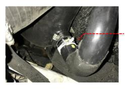
12 Check all hose clamps are secure. Test drive the vehicle to ensure vehicle performs correctly and there are no leaks/part interference during operation. Your installation is now complete!
