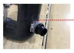
Place a 60-80 hose clamp on the turbo end of the Revo intake hose, and an 80-100 hose clamp on the airbox end. Push the Revo hose onto the turbo inlet and then onto the airbox making sure the hose sits flush.
