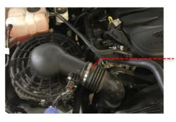
4 Using a 7mm socket, loosen the hose clamp that secures the intake pipe to the turbo. The intake pipe can now be removed from the vehicle.
