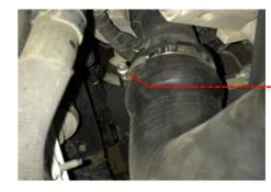
10 Use a 7mm socket tighten the hose clamp on the airbox end of the intake hose.
