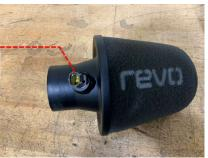
19 Install the front Revo intake hose onto the intake hard pipe using a 60-80 hose clamp, then insert the Revo air filter to the open end securing with another 60-80 hose clamp. When installing the Revo air filter ensure the temp sensor is positioned at an angle towards the rear of the heatshield so that the wire isn't over stretched. Check alignment and tighten both hose clamps, reattach the temp sensor connector.
