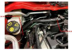
Remove the 10mm bolt on the intake pipe, unclip the wires from the pipe and then loosen the hose clamp at the base of the intake hose. Once this is done you can remove the intake pipe assembly from the vehicle, being careful not to catch any of the wires or pipes in the process.
