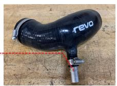
Bolt the Revo intake pipe bracket to the threaded hole, see step 7. Secure using the M6x50 bolt but don't fully tighten yet, to allow for alignment first.
