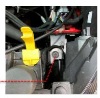
16 Install the Revo heatshield assembly by locating the dowels into the two rubber grommets, previously used by the OE airbox, and push down. Next bolt the heatshield bracket to the hole the 10mm bolt was removed from in step 15 using the M8x25 bolt and M8 washer.
