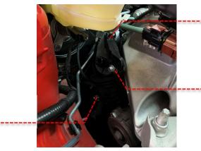
11 Install the breather hose connector into the Revo turbo intake hose, as shown, using the 12-22 hose clamp. Then install onto the turbo inlet pipe using a 60-80 hose clamp. Don't fully tighten yet, to allow for correct alignment first.
