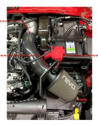
20 Reattach the two take-offs on the top of the hard pipe and then reconnect the breather pipe to the take-off on the turbo hose at the top of the engine.
