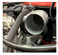
14 Assemble the Revo heatshield by first bolting the two steel mounting pins to the base of the Revo heatshield using the M8x16 bolts and M8 washers. Then install the heatshield bracket using the M6x16 cap head bolt, 2 x M6 washers and M6 nylock nut, as shown.
