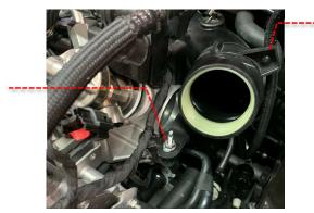
8 Move the coolant reservoir to one side to allow access to the lower intake hose. Do this by removing the tank off the two clips, shown, and place towards to the front of the engine.
