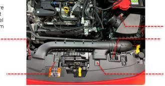
Remove the OE intake hard pipe by first unclipping the two take-offs on the back by popping the green clip out and then compressing the fittings to pull off.
