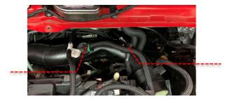
Next remove the 10mm nut at the front of the pipe along with the stud. Then remove the wire clips off the intake pipe.
