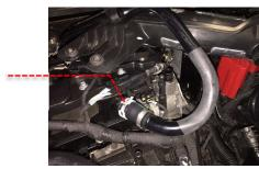
4 Unclip the third breather pipe from its nozzle and move to the right to help with installation.
