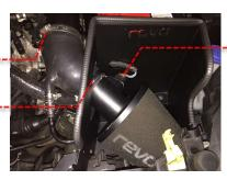
19 Install the heatshield bracket using the mounting point on the front slam panel using the OE bolt, as shown. Attach to the heatshield using the Móx16 bolt, Mó washers and Mó nylock nut.
