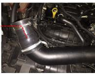
Take the long Revo breather hose and using the 25-35 hose clamp secure to the underside of the new intake pipe.
