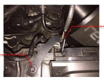
20 Reattach the breather pipe going over the intake pipe. Check that all hose clamps are tight and that everything is attached correctly and refit the engine cover. Test drive the vehicle to ensure vehicle performs correctly and there are no leaks/part interference during operation. Your installation is now complete!
