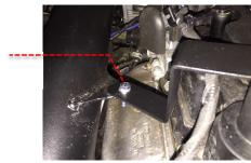
Assemble the secondary pipe bracket with the clamp, as shown. You will need to fully undo the hose clamp so you can slide it through the mini bracket assembly.
