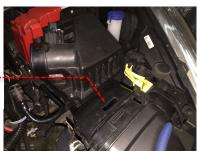
8 Unscrew the air flow sensor from the OE airbox and place safely to one side for use later in the installation.
