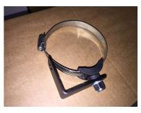
14 Install the assembled bracket to the side of the engine using a M6x16 bolt and M6 washer, as shown.
