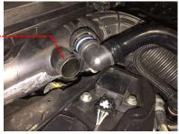
3 Remove the other end of the breather pipe from the front of the engine.
