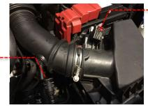
2 Unplug the second breather pipe from the breather nozzle found on the upper-rear of the engine
