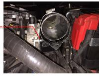
Install the new Revo elbow hose to the intake pipe through the hose clamp assembly. Loosely tighten the hose clamp and direct the Revo elbow hose downwards slightly. Install the small aluminium connector to the take-off on the hose using the 13-20 hose clamp. Ensure that the long part of the connector is in the silicone and the middle rim is offset from the edge of the silicone by about 3mm so the OE connector can clamp onto it.
