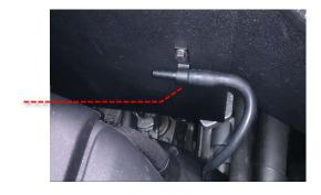
10 Install the Revo machined adapter into the turbo inlet. The Revo logo should face the turbo. Screw the adapter clockwise for 30° to 40° until it is secured.
