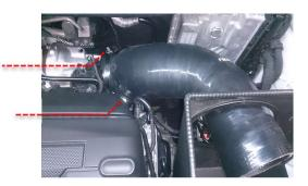
14 Using a 5mm hex key install the bracket to the Revo intake hose using the M6x12mm bolt and washer. With a 10mm socket refit the bolt from step 11 to secure the Revo bracket. Once everything is lined up on the bracket, tighten the hose clamp at the turbo.
