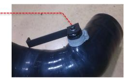
15 Connect the Revo vacuum hose from the connector to the intake hose. Install the Revo air filter using a 90-110 hose clamp. Check that all hose clamps are tight and that everything is attached correctly. Test drive the vehicle to ensure vehicle performs correctly and there are no leaks/part interference during operation. Your installation is now complete!
