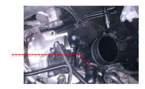
6 Insert the grommets, removed from the OE airbox in step 2, into the holes at the bottom of the Revo heatshield, as shown.
