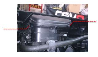
4 Using a T30 socket remove the bolt shown. Twist the turbo inlet elbow and remove from the turbo.
