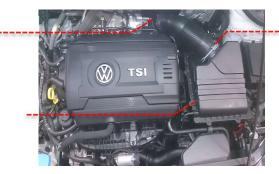
Pull the airbox upwards to detach from the rubber mounts. In the bottom of the airbox there are 4 x rubber grommets. Gently remove the 3 highlighted grommets from the airbox. Set aside, they will be reused later.
