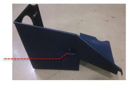
8 Secure the Revo heatshield in the OE airbox mounting grommets by pushing down into place. Use one of the T25 torx bolts from step 3 to secure the front of the heatshield in the position of the OE air intake.
