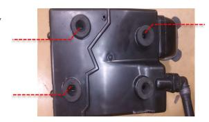
3 Using a T25 socket, remove the 2 x bolts that secure the front air intake. Keep the bolts as they will be reused later.
