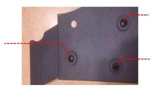
Using 2 x M5 washers, a M5x15mm bolt and a M5 nylock nut screw the vacuum connector to the side panel of the Revo headshield, as shown.
