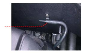
Install the Revo machined adapter into the turbo inlet. The Revo logo should face the turbo. Screw the adapter clockwise for 30° to 40° until it is secured.
