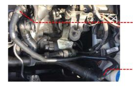
10 Insert the grommets, removed from the OE airbox in step 2, into the holes at the bottom of the Revo heatshield, as shown.
