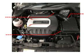
Pull the airbox upwards to detach from the rubber mounts. In the bottom of the airbox there are 4 x rubber grommets. Gently remove the 3 highlighted grommets from the airbox. Set aside, they will be reused later.
