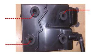
3 Using a T25 socket, remove the 2 x bolts that secure the front air intake. Keep the bolts as they will be reused later.
