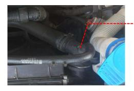
8 Clean and lightly grease the exterior of the check valve. Spray a small amount of lubricant inside the end of the Revo hose, as shown. Insert the check valve into the Revo hose, ensuring it is installed in the same orientation as the OE hose. Ensure the check valve stops at the approximate position, as shown, inside the Revo hose.
