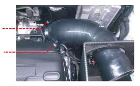
Using a 5mm hex key install the bracket to the Revo intake hose using the M6x12mm bolt and washer. With a 10mm socket refit the bolt from step 15 to secure the Revo bracket. Once everything is lined up on the bracket, tighten the hose clamp at the turbo.
