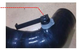
Connect the Revo vacuum hose from the connector to the intake hose. Install the Revo air filter using a 90-110 hose clamp. Check that all hose clamps are tight and that everything is attached correctly. Test drive the vehicle to ensure vehicle performs correctly and there are no leaks/part interference during operation. Your installation is now complete!
