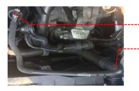
Remove the plastic check valve from the OE hose. Take note of the orientation of the check valve in the hose, it will need to be installed into the Revo hose in the same configuration.
