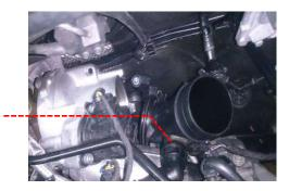
Ensure the vehicle coolant is cold. Remove the coolant reservoir cap slowly to relieve any pressure left in the coolant system. Loosen the hose clamp and disconnect the OE hose from the metal hard pipe in the area shown. Insert the cap (supplied) over the metal pipe and repeat at the radiator pipe end.
