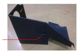
Secure the Revo heatshield in the OE airbox mounting grommets by pushing down into place. Use one of the T25 torx bolts from step 3 to secure the front of the heatshield in the position of the OE air intake.
