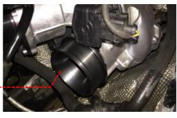
6 Remove the MAF housing from the OE airbox by removing the 2 x T25 torx screws holding it in place.
