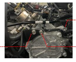
8 Install the MAF housing to the MAF bracket using the supplied M6x20 cap head bolts, M6 washers and M6 nylock nuts in the orientation shown.
