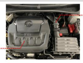
Remove the intake hose by loosening the jubilee clamp and tension clamp. Pull off PCV pipe from turbo elbow.
