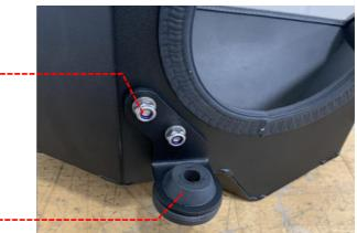
11 Install heatshield in car by pushing the rubber grommets onto locating pins you removed airbox from. Next install the front bracket by removing the T30 screw at the front and bolt the bracket to the same position, then attach to heatshield with the M6x16 cap head, M6 washers and M6 nylock nut.
