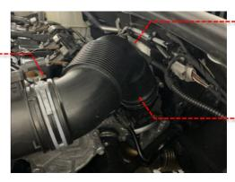
3 Undo the T30 on the turbo elbow and turn clockwise around 45\* and remove. Pull out T30 screw as no longer required.
