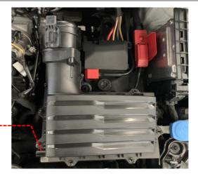
5 Install the Revo machined turbo inlet, first ensuring the o-rings are seated in the grooves in the neck. Locate onto the tabs on turbo and twist into place
