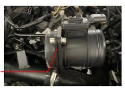
Install the machined PCV adapter in the Revo intake hose using the 25-40 hose clamp. Next install to the machined turbo inlet and MAF housing using supplied 70-90 & 60-80 hose clamps.
