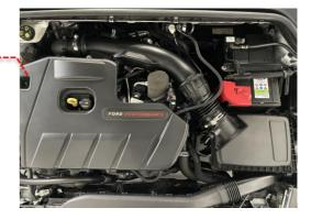
2 Remove the OE intake pipe, loosen the 2 x hose clamps then unclip the front breather pipe and DV hose to the rear. Finally remove the 2 x 8mm bolts on the bracket and pull away from turbo hose and airbox.
