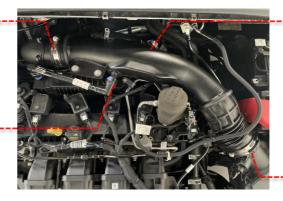
3 Remove the OE turbo inlet pipe by loosening the hose clamp at the turbo end.
