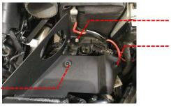
Install the Revo intake hard pipe and secure using the hose clamp fitted to the Revo intake hose, as shown.
