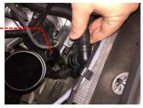
Remove the T30 bolt attaching the turbo inlet pipe to the turbo, then twist the inlet pipe and remove.
