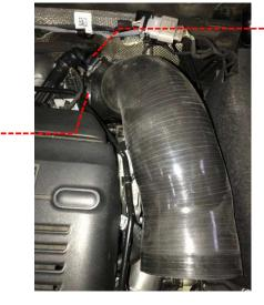
Assemble the mini bracket assembly onto the 90-110 hose clamp and attach the pipe bracket, as shown.
