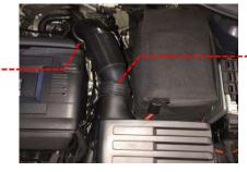
2 Disconnect the breather pipe from the turbo inlet.
