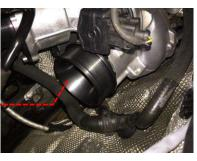
Pull the vacuum pipe off the side of the airbox lid and pull upwards on the airbox assembly to release from the rubber grommets, remove from the vehicle.
