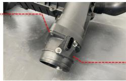
6 Assemble the Revo heatshield bolting the heatshield bracket to the base using the supplied M6 bolts, washers and nylock nuts as shown. Then insert the VW OE rubber gromets into the hole on the bracket and base of heatshield.
