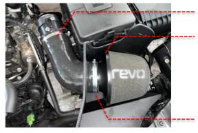
10 Install the connecting silicone hose to the MAF and then the hard using the remaining 70-90 hose clamps. Re-connect the MAF wire and check all clamps are secure.
