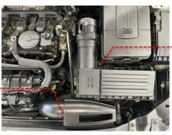
4 Remove the front duct by removing the 2 x T25 torx screws (retain for later use).
