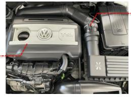
Remove the back pipe by first removing the tension clamp on the MAF housing and at the Turbo, then remove the T30 bolt on the rear bracket (retain for later use) before finally disconnecting the breather pipe from the pipe. Ensure the rubber hose on the turbo is removed so that you are installing directly onto the turbo inlet later.
