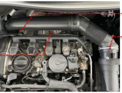
3 Next remove the airbox assembly by loosening the 6mm allen bolt at the back of the box and unclip form the front duct. You should then be able to pull up on the airbox to remove from rubber mounting points.
