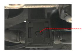
Disconnect the MAP sensor located on the throttle hard pipe.
