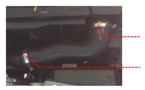
Check the clearance of the Revo discharge hard pipe to the radiator fan shroud. If less than 5mm, adjust the discharge turbo silicone hose and hard pipe until a minimum clearance of 5mm is achieved. Once adequate clearance has been obtained at this point and at step 17, tighten all the hose clamps. Tighten the upper discharge pipe mounting bolt to 35Nm.
