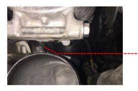
27 Install the coolant hose and wiring harness clips onto the Revo brackets.
