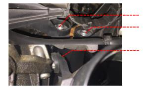
10 Unclip the wiring harness from the mounting on the discharge pipe by pressing the tab, shown, and pulling the harness downwards.
