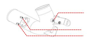
Install the Revo throttle hard pipe onto the Revo hose. Bolt the Revo throttle hard pipe to the block using the M6x16mm bolt and M6 washer supplied, as shown. Note: ensure the supplied rubber washer is used between the Revo pipe bracket and block (not shown). Do not fully tighten the bolt at this time.
