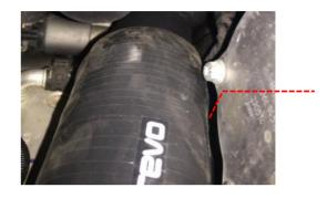
Reclip the wiring harness retaining clip to the upper bracket on the Revo discharge pipe. Install the coolant hose retaining clip onto the lower bracket and corresponding coolant hose. Refit the wiring harness mounting clip to the starter bracket.
