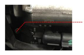
From the underside of the vehicle use a 7mm socket to loosen the 4 x intercooler hose clamps and remove the intercooler hoses.
