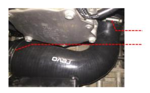
Align the bracket on the Revo discharge hard pipe with the corresponding threaded hole on the cylinder head bracket. Install the supplied rubber washer between the threaded bracket and the Revo hard pipe. Loosely install the M6 bolt and washer. Do not tighten the bolt at this time.
