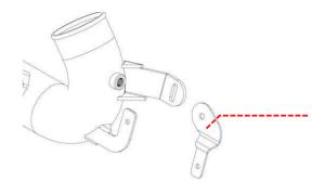
Align the Revo throttle hard pipe until there is a minimum clearance of 6-7mm between the top of the pipe and the underside of the air conditioning compressor. Once the clearance has been achieved tighten the bolt to 30Nm.
