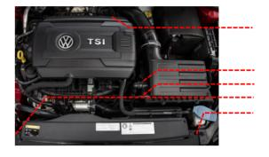
2 If fitted, unclip the gearbox breather from the battery tray and set aside.
