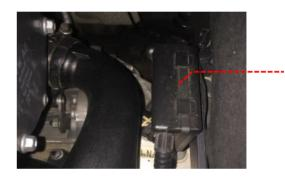
3 Using a 7mm socket loosen the 2 x clamps on the discharge turbo hose.
