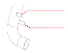
Reinstall the intercooler discharge hose.
