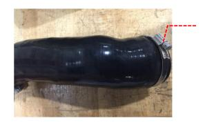
Install the Revo throttle hose ensuring the section with the internal step, as shown, is inserted onto the throttle body. Align the Revo hose within the engine bay until the Revo hose has a minimum 1-2mm clearance to all surrounding parts. Install the remaining 60-80 hose clamp onto the bottom of the Revo hose.
