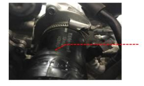
Remove the discharge hard pipe from the top of the engine bay and remove the coolant hose clip (if fitted). Set aside, out of the work area.
