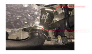
4 Using a T30 socket loosen the bolt mounting the discharge hard pipe to the engine head bracket.
