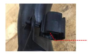
7 Using a 7mm socket, loosen the hose clamp holding the throttle pipe to the throttle body.
