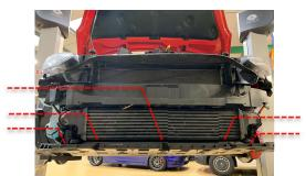
8 Remove the top plastic shroud by loosening the 4 x cross head clips then unclip the air temp sensor from the shroud before removing from the vehicle. Then simply unclip the lower shroud from the crash bar and remove.
