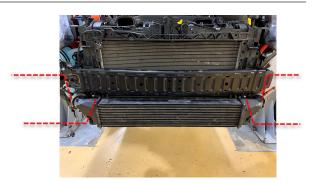
10 Remove the 2 x 13mm bolts holding the lower intercooler brackets in place and keep the bolts and grommets to one side. Then remove the 2 x 10mm bolts above the crash bar and keep with the others you just removed.
