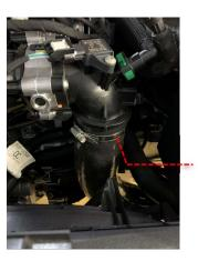
19 Bolt the new temp sensor bracket to the plastic surround using the supplied M6x16 self-tapping bolt. Then attach the temp sensor to the bracket pushing it through the holes.
