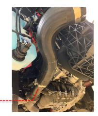
12 Remove the front intake by removing the 2 x T30 bolts holding it down and unclipping the rubber hose on top. Note: the air filter set up you are running may change this step slightly.
