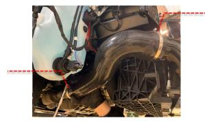
18 Install the new Revo throttle hose by sliding the hose clamps over each end, 50-70 on the throttle body end and 60-80 on the intercooler end. Then push the hose up onto the throttle body and then onto the Revo intercooler, secure each clamp once in position.
