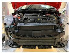
6 Unclip the bumper from each arch and then pull away from the vehicle.
