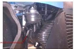
7 Disconnect the air temperature sensor from the OE intercooler. Using an 8mm socket unscrew the 2 x bolts, at the bottom of the intercooler and remove the intercooler.
