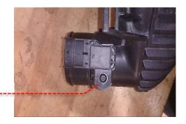
9 Secure the temperature sensor to the Revo intercooler using a M4x10mm hex key bolt and a M4 washer.
