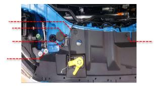
Remove the two air guides by pulling them gently. Remove the two remaining plastic covers by pulling them downwards.
