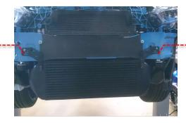
12 Use 2 x M6x20 bolts, 4 x M6 washers and 2 x M6 nylock nuts, to secure the Revo intercooler to the OE mounting points, with a 10mm socket and a 10mm spanner. Reconnect the air temperature sensor and tighten the intercooler hoses using a 7mm socket.
