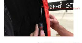
6 Remove the bonnet release handle by pushing the release button, found at the 12 o'clock position, and pulling up on the handle.
