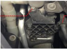
1 Unplug the sensor from the coolant tank and then remove the 2 x T25 screws holding the tank to the chassis. Next unclip the coolant line and lift the tank out of the chassis and secure out of the way.
