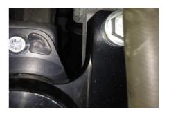
Reinstall the washer filler neck bracket you removed earlier. If your vehicle is not equipped with a noise pipe or charcoal canister, install the Revo accessory bracket spacer between the washer filler neck bracket and Revo accessory bracket. Install both the washer filler neck bracket bolts loosely, then tighten the bolt on the mount to 57Nm with a 15mm socket. Lower and remove the hydraulic jack.
