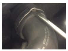
D Using tension clamp pliers slide the hose clamp back and remove the noise pipe from hose.
