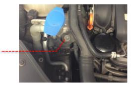
Using a flat head screwdriver remove the noise pipe from the firewall coupling by prying the clip upward and removing from the plastic groove. Remove the coolant lines from the clamps on the side of the pipe.
