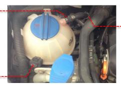
2 Using a 10mm socket remove the bolt holding the washer filler neck to the filler neck bracket.
