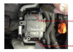
5 Using an 18mm socket remove the two bolts that hold the mount to the engine. Note: you will need to gently move and hold the three coolant hoses out of the way to get to the bolts.
