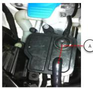
B Loosen the T30 bolt holding the noise pipe to the engine mount. The bolt is captive and will not remove from the bracket.
