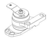
7 Install the Revo engine mount in the engine bay and bolt loosely into position using 2 x M10 chassis bolts and 2 x M12 engine bolts. After all 4 x bolts are loosely installed, position the Revo mount arm as shown and then tighten the M12 bolts to 60Nm using a 19mm socket then tighten the M10 chassis bolts to 46Nm with a 15mm socket.
