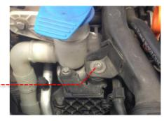
F Unclip the hose from the composite bracket, then using a 10mm socket remove the nut and bolt supporting the bracket.
