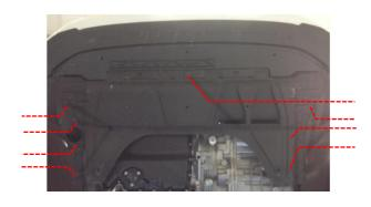
Using a hydraulic jack with a suitable piece of wood on it, carefully support the engine from underneath. Position the jack so that it won't cause any damage. Note: the engine sump is composite and more fragile than a steel sump.
