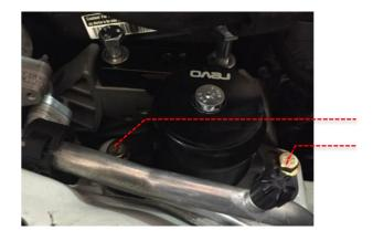
11 Ensure the Revo mount arm is aligned parallel with the edge of the engine block bracket. Keep the arm in this position and use a 19mm socket to torque the bolts to 60Nm.
