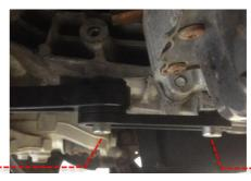
Torque the M14 bolt on the rubber subframe mount to 100Nm. The Revo bush should be touching the base of the rubber subframe mount. Refit all OE parts back to vehicle. Reinstallation is the reverse of removal. Follow any factory torque specification during reinstallation of OE parts. Test drive the vehicle to ensure there are no leaks/part interference during operation. Your installation is now complete!
