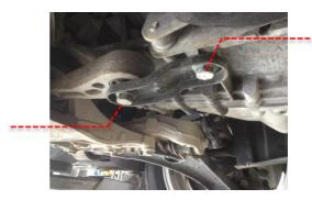
4 Using some white lithium or red grease, heavily grease all the walls of the three Revo insert uprights to ease insertion. Note: TFSI insert pictured, TSI insert is installed the same way.
