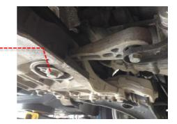
3 Using a 16mm socket remove the two bolts that couple the torque mount link and bracket to the transmission. Remove both the torque mount arm and link bracket.
