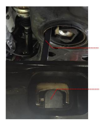
Insert the Revo installation tool, as shown. Note: now the socket head cap screw inserts through the thin, unthreaded washer and threads into the handle, now positioned at the top of the subframe. Also, note the orientation of the handle relative to the OE torque arm. Using an 8mm hex key tighten the socket head cap screw until the OE mount aligns with the subframe window, as shown.
