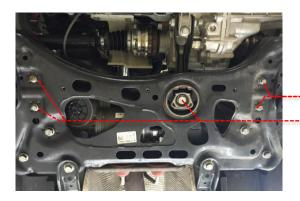
3 Using a 16mm socket, remove the 2 x bolts fixing the aluminium torque mount to the gearbox. Remove the OE torque mount arm assembly and set aside.
