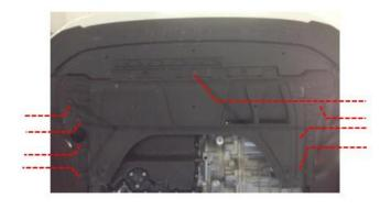
Using a hydraulic jack with a suitable piece of wood on it, carefully support the gearbox from underneath. Position the jack so that it won't cause any damage. Note: the cast gearbox case can crack easily.
