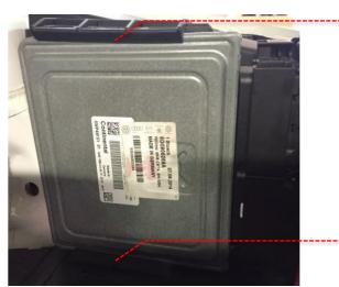
9 Using a 10mm socket, remove the 2 x nuts securing the engine control unit holder. Remove the holder and set it aside.
