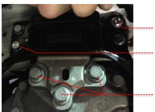
12 Check the pre-assembled Revo mount to ensure the arm can rotate within the bushes.
