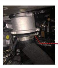
3 Remove the 3 x bolts on the muffler and then remove the OE part from the turbo.
