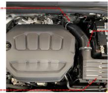
Next, loosen the hose clamp securing the discharge hose to the OE muffler and discharge pipe and remove. You may need to loosen the discharge pipe if this is too tight by removing the T30 bolt on the pipe.
