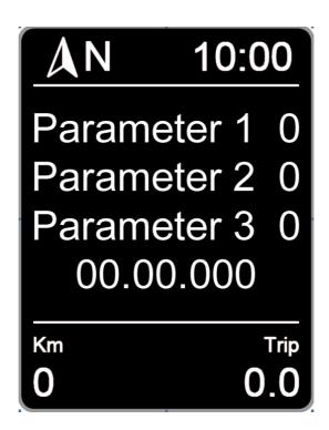
NOTE: As you can see in the picture, the counter displays instead of the 4<sup>th</sup> data parameter when the stopwatch function is activated. You can still switch between the set number of data parameter screens.
