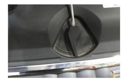
2 Remove the slam panel by unclipping along the front edge and then sliding it out from under the front air scoop.
