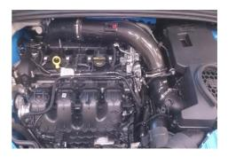
9 Check that there is ~3-5mm of clearance between the bonnet shrouding (fabric material) and the top of the carbon pipe there is ample (>2mm) clearance around all engine parts. Reinstall the vacuum line. Tighten all hose clamps (turbo hose clamp, carbon pipe hose clamp, air box hose clamp) using a 7mm socket. Reinstall the engine cover. Your installation is now complete, GO PLAY!
