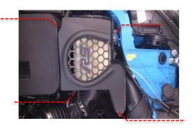
Install the Revo air filter into the OE airbox by aligning the metallic flange with the corresponding points on the OE airbox.
