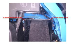
Remove the engine cover by pulling up and off the rubber mounts. Remove the (2) intake pipe bolts using a 10mm spanner. Remove the (4) OE hose clamps on the intake pipe using a 7mm socket. Unclip the vacuum line on the OE intake pipe and remove the pipe.
