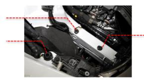
4 Remove the OE filter from the airbox and then remove the inner plastic plate in the front section of the airbox by removing the two self-tap screws using a T25 bit as shown.
