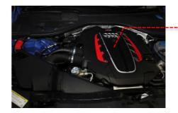
2 Loosen the 2 hose clamps on the two intake pipes using a 7mm socket and remove.
