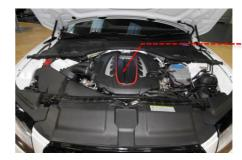
2 Loosen the 4 hose clamps on the two intake pipes using a 7mm socket and remove.
