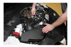
3 Unclip the front intake duct from the airbox, then pull up on the airbox to remove from the rubber mountings. Ensure you leave all three of the rubber mountings in place as they will be reused.
