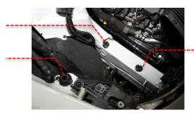
4 Install the new Revo filter onto the new intake pipe and then clip into the new RS airbox.
