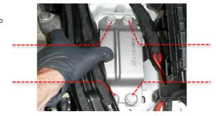
10 Ensure that the Revo transmission mount is assembled in the correct configuration as shown. Loosen the flat head socket cap screw with a 6mm allen key so you can rotate the arm to position correctly.
