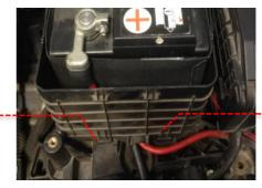
5 Remove the three newly exposed battery tray bolts with a 10mm socket.
