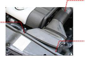
Unclip the MAF senor and secure out of place so as not to damage. Next if the car has a secondary air injection, unclip from front section. Remove the two T25 torx screws holding the front scoop in place. Remove the 5mm allen bolt which hold the airbox to the battery tray. Finally using tension pliers remove the back pipe off the MAF housing and pull the airbox assembly out and place to one side.
