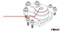
Sit the Revo transmission mount into the cavity and install using the three supplied M12 bolts and four supplied M10 bolts into the transmission/chassis threaded locations. With another person align the Revo mount arm to the position shown on the right. Pull the engine forward and tighten the M12 bolts with a 19mm socket to 44 ft.lbs once correctly aligned.
