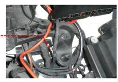
7 Using a hydraulic jack with a piece of wood on it, gently support the transmission from the bottom. Ensure that you do not damage the composite splash tray, then raise it by about 3mm form its current position. Using an 18mm socket remove the three bolts that hold the transmission to the OE mount.
