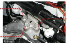
Using a medium sized flat screwdriver, gently pry between the chassis and the plastic wiring cage to free from the chassis.
