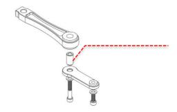
8 Check that the Revo torque arm protrudes through the centre of the subframe provision. Adjust accordingly if required then torque the two socket head bolts to 30 ft.lbs.
