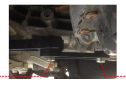
Once everything else is installed, torque the M14 bolt on the rubber subframe mount to 74 ft.lbs. The insert should be touching the base of the rubber subframe mount. Check the other bolts are torqued accordingly and remove the vehicle from the ramp or jacks and test drive. Your installation is complete. GO PLAY!
