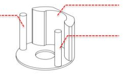
Place the insert into the corresponding locations on the OE rubber subframe mount. The back edge of the Revo insert should be parallel with the steering rack during installation. It is useful to use a hydraulic jack with a block of wood at this point to apply constant pressure to the base of the insert until it sits flush with the bottom of the rubber subframe mount.
