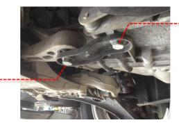
4 Using some white lithium or red grease, heavily grease all the walls of the three Revo insert uprights to ease insertion. (Note: FSI insert pictured, TSI is insert installed the same way)
