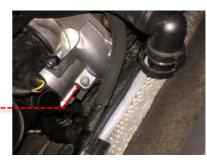
4 Install the new machined Revo turbo inlet. Note: It will only fit onto the turbo one way so you wil need to line up the slots on the inlet to the turbo first, once lined up push into the turbo and then twist 90° so it locks into place.
