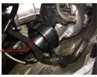
Insert the aluminium breather adapter into the new hose and secure using the 25-35 hose clamp. Next Install the new revo upgraded hose using the two 70-90 hose clamps, start by slipping over the turbo inlet then onto the airbox lid and secure.
