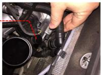
Remove the T30 bolt attaching the turbo inlet pipe to the turbo, then twist the inlet pipe and remove from the car.
